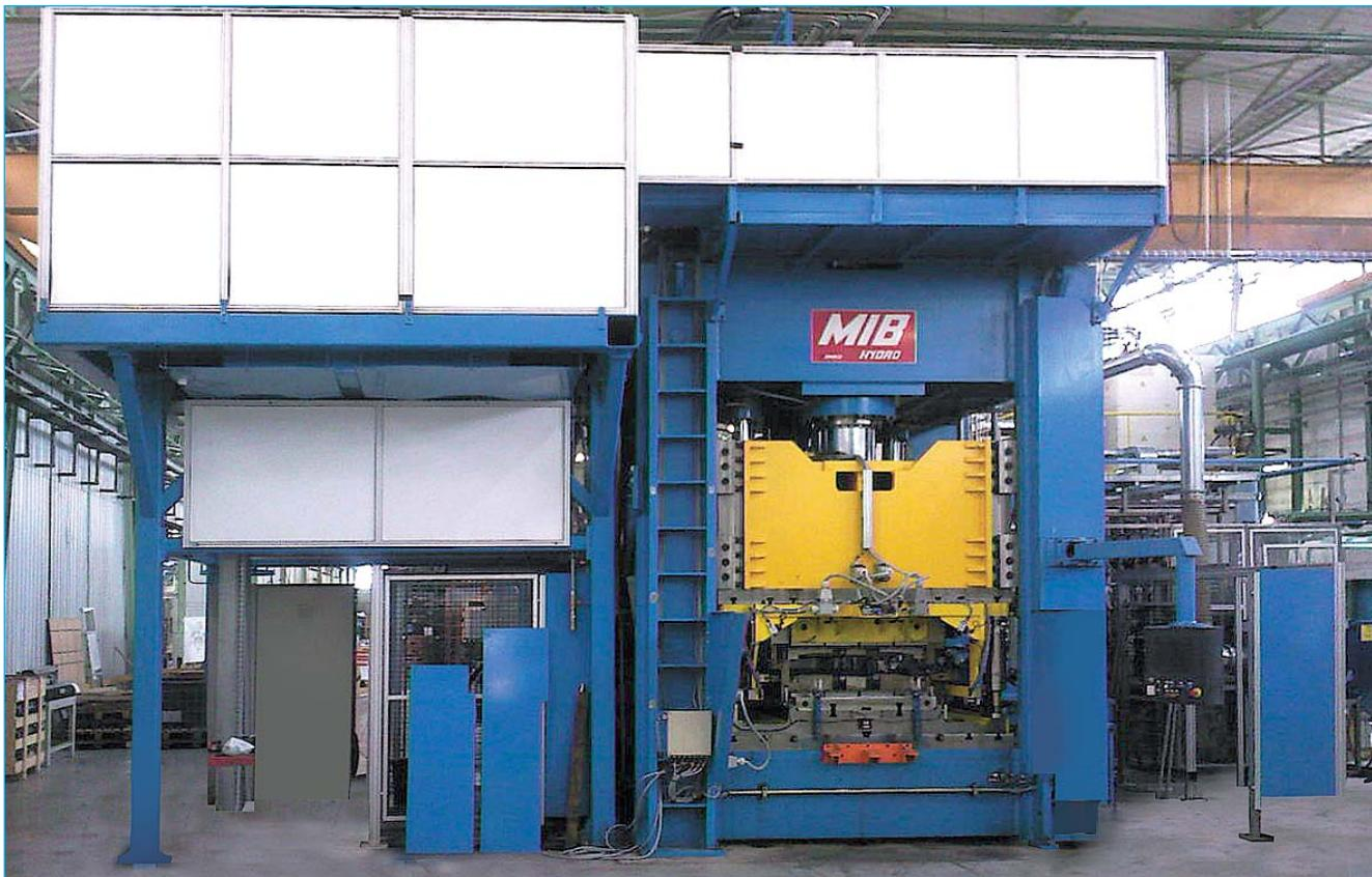
This 1000 T arch press manufactures tubes using a multi-steps tool.
